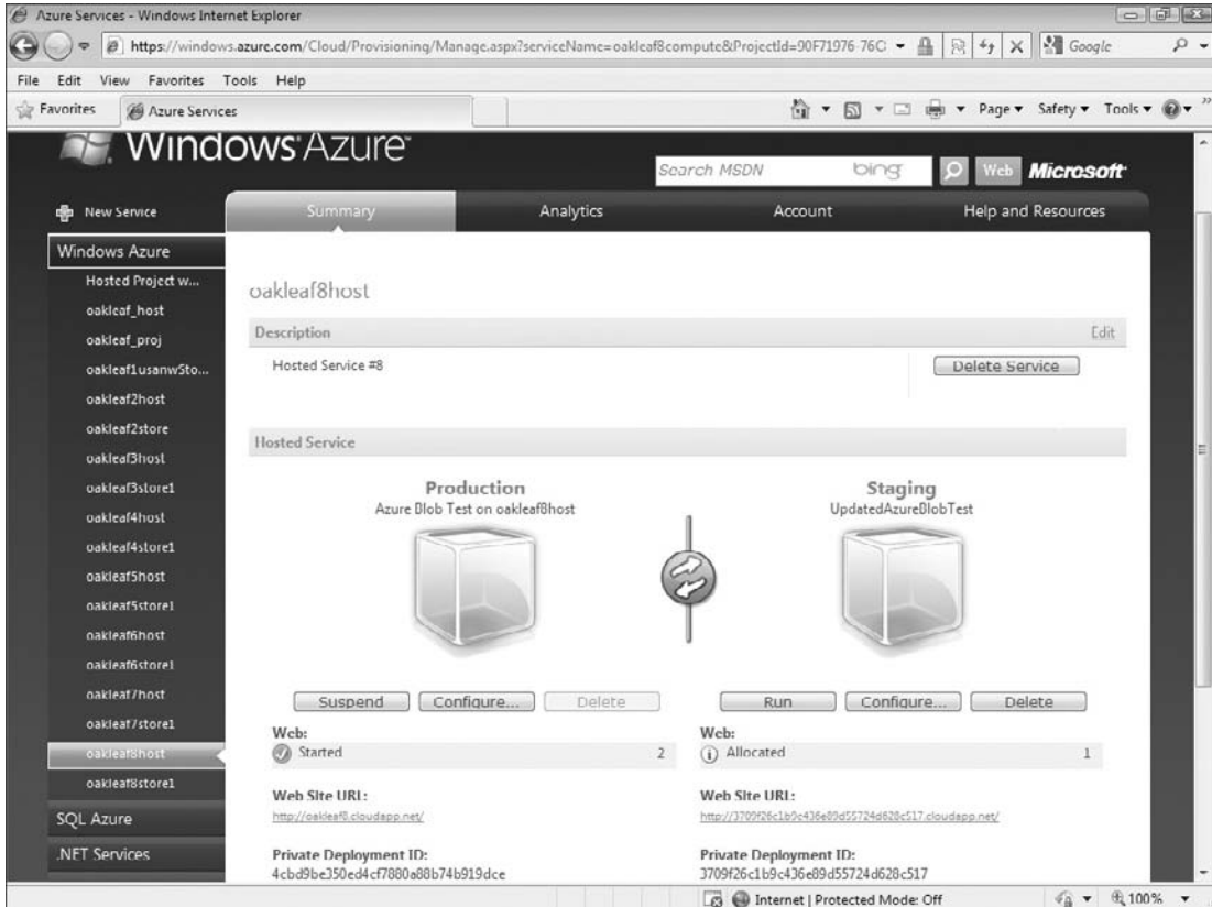
Figure 2-19: After deploying your project to the Staging service, click Run to place it in the Started role and then click the Web Site URL link to test it under the Windows OS operating system.
