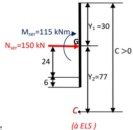
$$\beta_1 = 0.893 \text{ et } k_1 = 31.73 \quad \text{d'où} \quad A_f = \frac{M_1}{\beta_1 d \sigma_s} = 6.83 \text{ cm}^2$$
