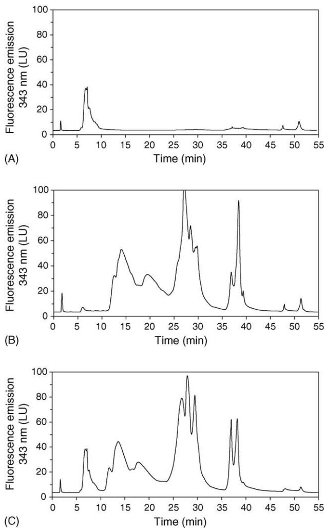
Fig. 2. HPAEC intrinsic fluorescence chromatogram of 100  $\mu\text{g/ml}$  EPO BRP (A), 3 mg/ml HSA (B) and 100  $\mu\text{g/ml}$  EPO BRP containing 3 mg/ml HSA (C).
