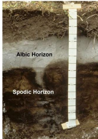
An albic horizon (white) above a spodic horizon (dark brown) in a snail in New Zealand. Scale is in cm.
