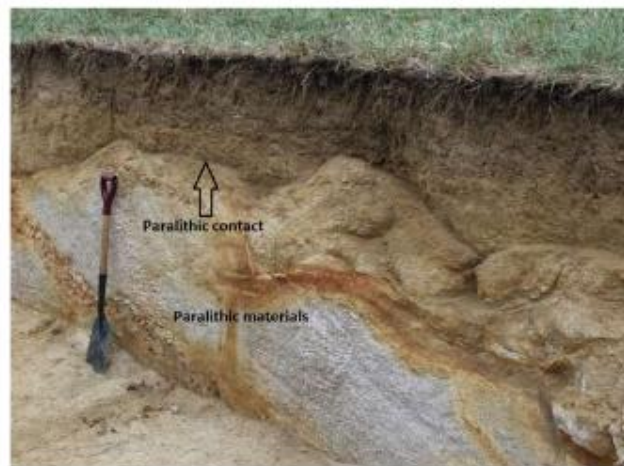
This soil has an abrupt way boundary at the paralithic contact. The material below the contact is relatively soft, weathered bedrock that can be dug with a spade. (Photo courtesy of John Kelley)
