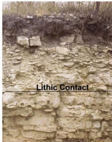
Soil profile with a lithic contact over hard limestone. Note that the upper part of the profile consists of soil and loose rock fragments. The lithic contact is at the top of the continuous bedrock layer, which comprises about the lower third of the photo.
