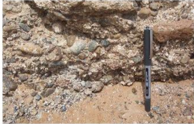
Old alluvial gravel cemented in a matrix of illuvial calcium carbonate (white) form a very strongly cemented petrocalcic horizon (in a soil in the United Arab Emirates). (Photo courtesy of Dr. Craig Ditzler)
