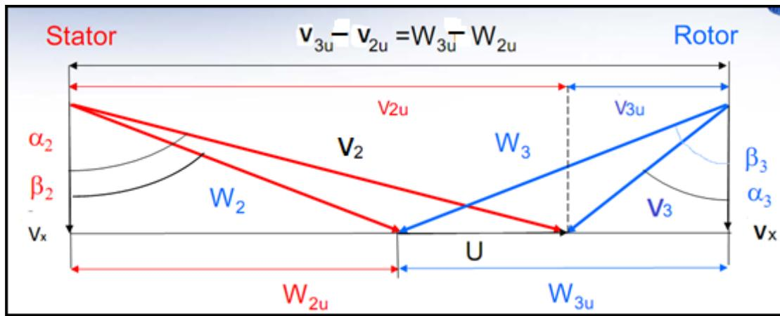
$$W_e = U(V_{3u} - V_{2u})$$
