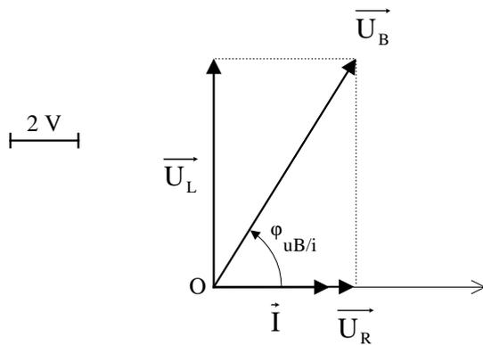
$$U_R = U_B \cos \varphi_{uB/i} = 4,25 \text{ V}$$
