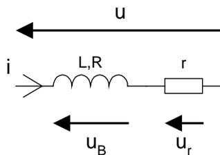
On donne  $f = 50 \text{ Hz}$ ,  $U = 14 \text{ V}$ ,  $U_B = 8 \text{ V}$  et  $U_r = 8 \text{ V}$ .
