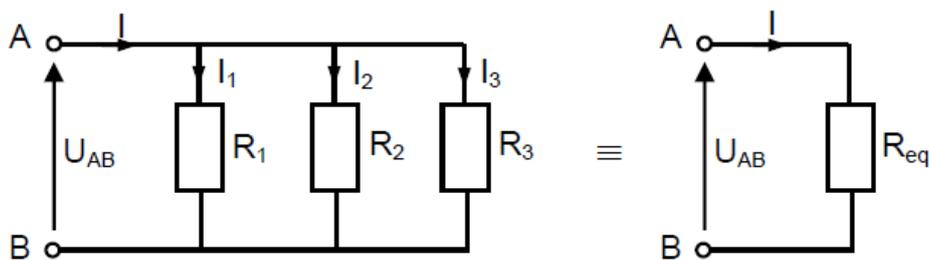
$$I = I_1 + I_2 + I_3 = \frac{U_{AB}}{R_1} = \frac{U_{AB}}{R_2} = \frac{U_{AB}}{R_3} \Rightarrow U_{AB} = I \left( \frac{1}{R_1} + \frac{1}{R_2} + \frac{1}{R_3} \right) = I \cdot R_{eq}$$
