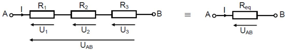
$$U_{AB} = U_1 + U_2 + U_3 = R_1 \cdot I + R_2 \cdot I + R_3 \cdot I = I \cdot (R_1 + R_2 + R_3) = I \cdot R_{eq}$$
