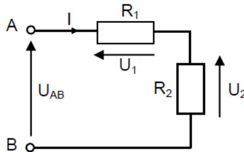
$$\bullet U_2 = R_2 \cdot I = R_2 \frac{U_{AB}}{R_1 + R_2}$$
