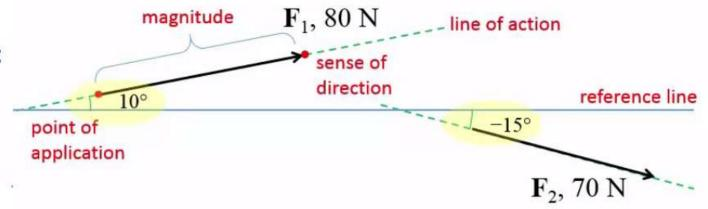
The direction of a force can be descibed by the angle made by its line of action and a reference line.
