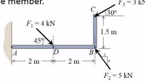
Example: Determine the total moment about point  $\bf A$  caused by the three forces  $F_1$ ,  $F_2$  and  $F_3$ . Take counterclockwise as positive.
