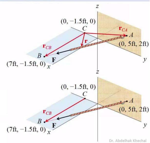
Question 2: If force F has magnitude of 450 N and is directed from point A to B as shown, determine the moment (Cartesian vector form) caused by **F** about point O.
