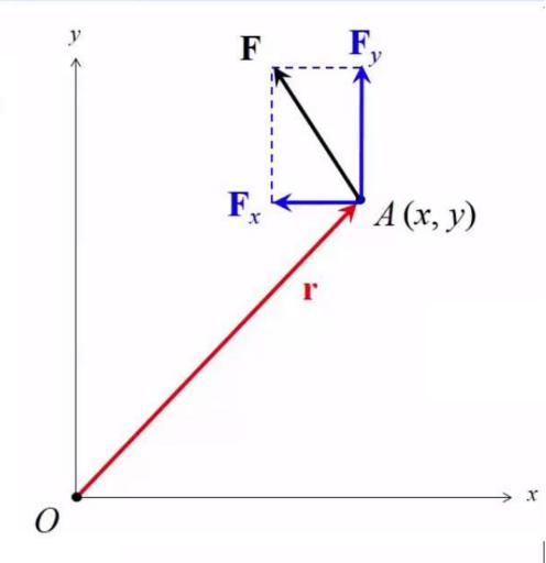
Sometimes, we can conveniently resolve the force into one component that is **along** the direction of **r** pointing from *O* towards *A*, and another component that is **perpendicular** to **r**.
