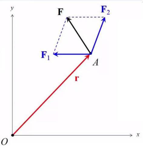
The moment caused by a force can be calculated by summarizing the moments caused by its component forces about the same point and this is the Principle of Moments.
