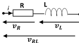
$$v_{RL}(t) = v_R + v_L = V_{eff\ R-L} \sqrt{2} \sin(\omega t + \varphi) \quad (**)$$
