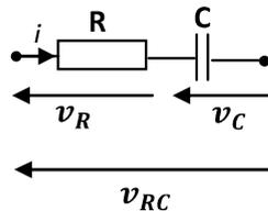
$$v_{RC}(t) = v_R + v_C = V_{eff R-C} \cdot \sqrt{2} \sin(\omega t + \varphi_{RC})$$
