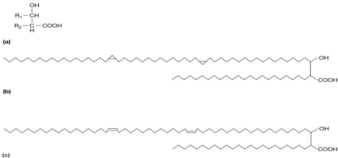
**Figure :** Mycolic Acid Structure. (a) The generic structure of mycolic acids, a family that includes over 500 different types. (b) A mycolic acid with two cyclopropane rings and (c) an unsaturated mycolic acid.
