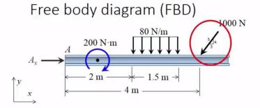
We see that there is a **horizontal component** of this force that will **push** the member to the **left**. Therefore, the wall must exert a horizontal force to the **right** to prevent this motion to the **left**.
