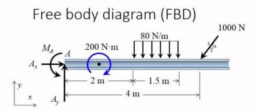
Finally, the forces and **the moment** all cause the member to **rotate** clockwise. Therefore, the wall also must exert **a moment support** that is **counterclockwise**, in order to prevent this **rotational motion**.
