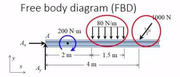
Because of the vertical component of the **concentrated force**, as well as **the distributed force**, causing the member **to go down**. Therefore, the wall must exert **a vertical force up** in order to prevent this downward motion.
