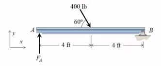
A **roller is similar to a rocker**, or **a simple contact** support. It exerts a force that is perpendicular to the contacting surface.
