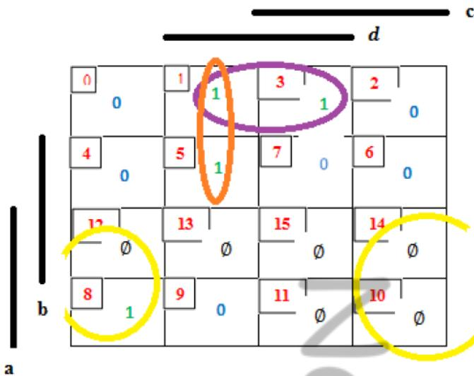
$$D = a\bar{d} + \bar{a}\bar{b}d + \bar{a}d\bar{c}$$
