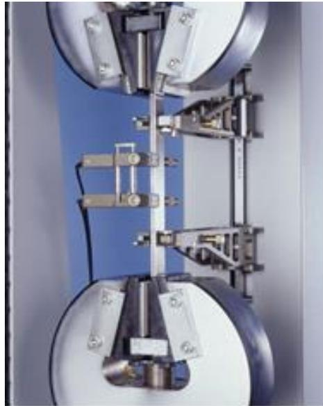
Figure 4 :Taste de traction
