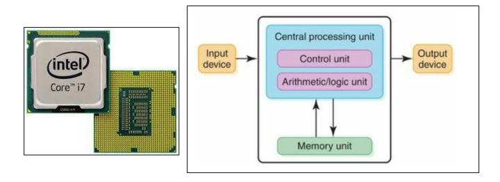
The central processing unit or the microprocessor is the physical heart of the entire computer system. It is composed of:
