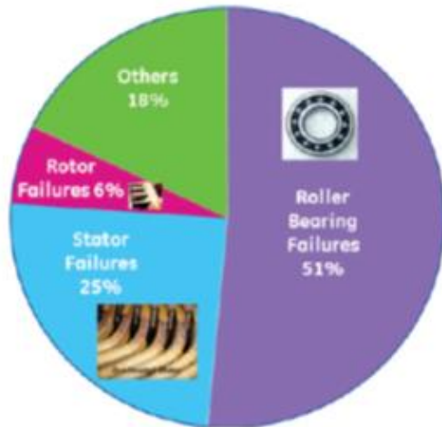
Figure 15 - Failure modes for typical AC motors up to 4 kV (REB)
