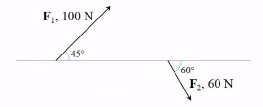
Example 1: What this the magnitude and direction (with respect to the horizontal reference line) of the resultant force of  $\mathbf{F}_1$  and  $\mathbf{F}_2$ ?
