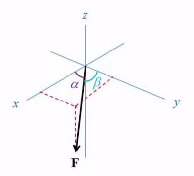
Question 3: If the coordinate direction angles  $\alpha = 112^{\circ}$ ,  $\beta = 75^{\circ}$  and  $A_z = 5.0$  cm, determine the magnitude of vector **A**.
