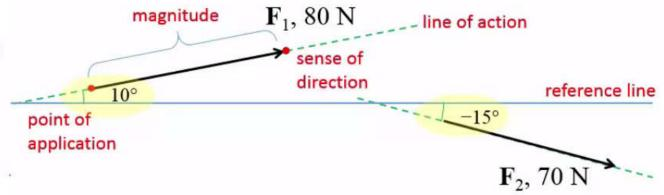
The direction of a force can be descibed by the angle made by its line of action and a reference line.
