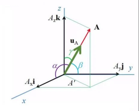
"The cosine squared of the three coordinate direction angles for any Cartesian vector must equal 1."
