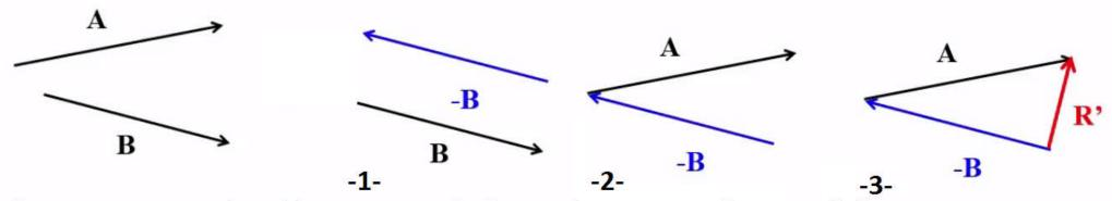
Then, we can simply add vector A to (-B) together using either Parallelogram Low or Triangle Rule.
