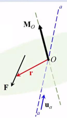
The direction of this moment is not necessarily along the (aa) axis as we want it
