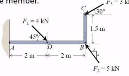
Example: Determine the total moment about point A caused by the three forces  $F_1$ ,  $F_2$  and  $F_3$ . Take counterclockwise as positive.
