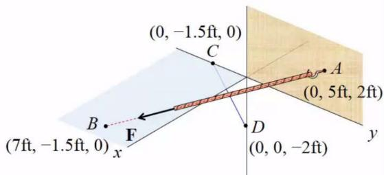
Example: The line of action of force  $\mathbf{F}$  directs from point A to point B. If the magnitude of the force is 120 lb, determine the magnitude of the moment caused by  $\mathbf{F}$  about the CD axis.
