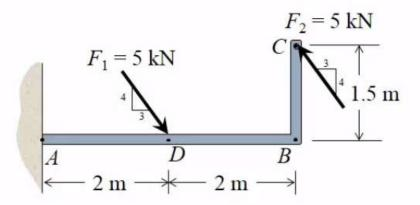
Example: Determine the magnitude of the applied couple moment. Neglect the thickness of the member.
