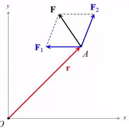
The moment caused by a force can be calculated by summarizing the moments caused by its component forces about the same point and this is the Principle of Moments.
