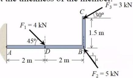
Question 2: Determine the total moment about **point** C caused by the three forces  $F_1$ ,  $F_2$  and  $F_3$ . Take counterclockwise as positive. Neglect the thickness of the member.
