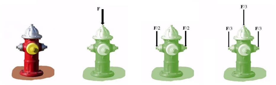
From experience, we can say that if we replace this force **F** by **two forces** (Fig.2), each **with half the magnitude**, placed **symmetrically** about the **central axis**, these two forces will create the same effect as the original **F** force. Even if we replace the forces by these three (Fig.3), again, they create the same effect.
