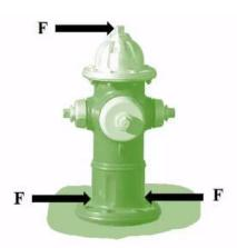
For this fire hydrant to **stay still**, as a response, the ground must **create a force** supporting the fire hydrant, pointing to the left, and also a moment to cancel out **the rotational effect**.
