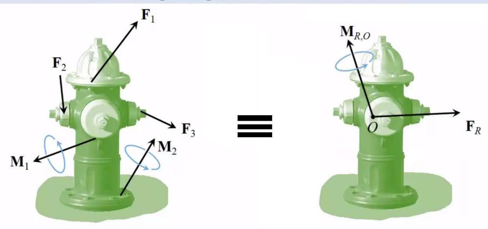
We replaced the original multi-force multi-moment load system by a single force single moment system.
