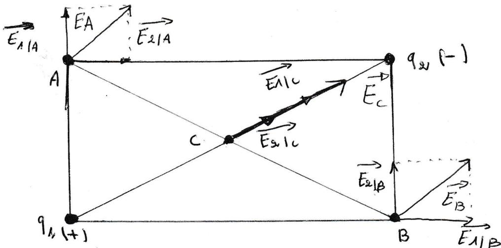
$$E_{1/B} = \frac{9 \times 10^9 \times 3,2 \times 10^{-11}}{(8 \times 10^{-2})^2} = 45 \text{ V/m}$$
