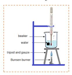
2. Take a measurement of the water temperature before you start heating the water.
