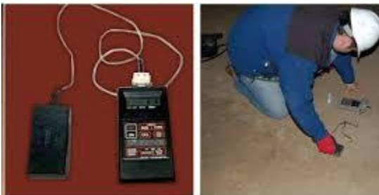
Pachometer is a non-destructive magnetic device used to locate existing rebars in concrete structures. Utilizing this equipment, FKC can determine the concrete cover, rebar sizes, spacing, and length.
