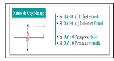
If  $\overline{OA} < 0$  the object is real If  $\overline{OA} > 0$  the object is virtual
