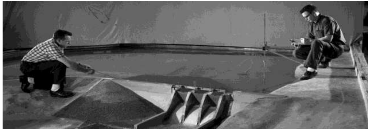
Tennessee Valley Authority civil engineers monitoring hydraulics of a Tellico Dam scale model.
