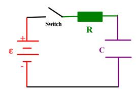
After the switch is closed the current is entering the capacitor so that I = dQ/dt, where Q is the charge on the capacitor and summing all the potential changes in going around the loop gives
