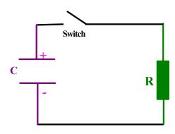
After the switch is closed the current is leaving the capacitor so that I = -dQ/dt, where Q is the charge on the capacitor and summing all the potential changes in going around the loop gives
