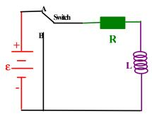
where I(t) is a function of time. If the switch is closed (**position A**) at t=0 and I(0)=0 (assuming the current is zero at t=0) then
