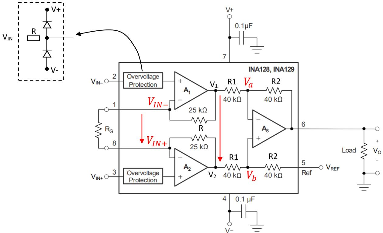
$$V_{IN+} - V_{IN-} = \frac{R_G}{R_G + 2R} (V_2 - V_1)$$
