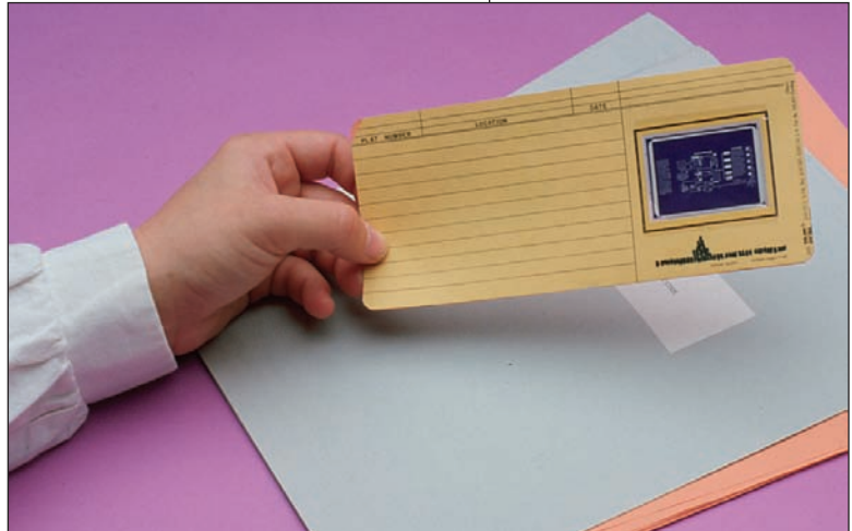
An aperture card has an opening designed as a carrier for film image(s).
