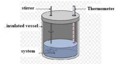
To measure the temperature inside the calorimeter vessel, we use a thermometer and a stirrer (agitator) to ensure homogeneous temperature within the vessel.
